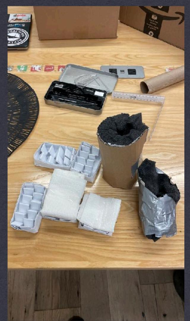
We experimented with different materials and we wrapped the egg around the foam and did a drop test. Egg survived.
